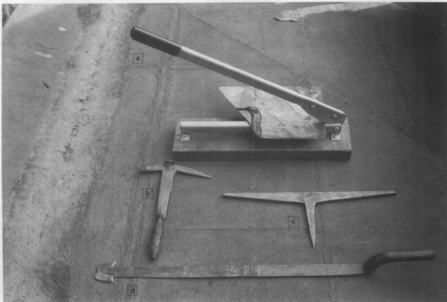
Figure 17. Slater's Tools. The cutter (a) is used to trim slate edges; the slate hammer (b) is used for hammering nails, trimming, cutting and punching holes in slates, and pulling roofing nails; the steak (c) is a T-shaped piece of iron upon which the slater places the edge of a slate to be trimmed; and the ripper (d) is slid under the slates to pull out the nails.
