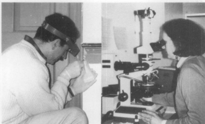
Figure 9. Conservators are shown in the two-part process of conducting a complete paint investigation: (a) Paint samples are carefully collected onsite. (b) In the laboratory, an ultra violet light microscope is used to identify pigment and binding media. Paint samples are photographed with the camera mounted on top of the microscope. (right). Photo left: Courtesy, Matthew J. Mosca; Photo right: Courtesy, Andrea M. Gilmore.
