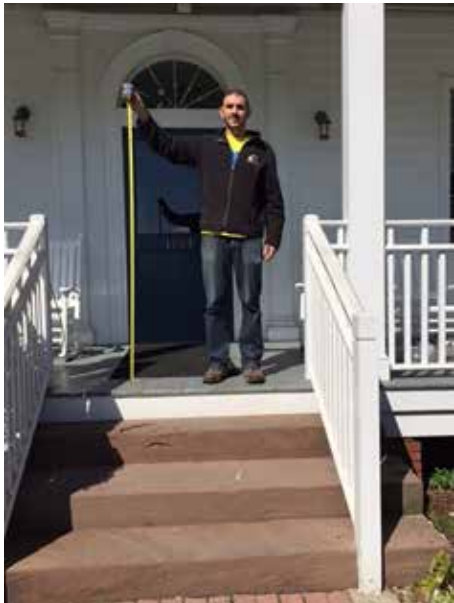
[81] When planning to elevate a building, it is helpful to create mock-ups or visual representations to illustrate the new floor height in comparison to the existing height in order to evaluate the impact on the historic character of the building. In this example, the proposal is to elevate the building to 6 feet above the existing first-floor level. Photo: Dianne Selditch/SoundWaters
